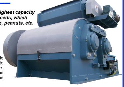
The heart of the hulling process is the twin, rugged 18" dia rolls equipped with removable huller knives. These twin rolls are driven at a ratio to enhance the cutting process thus minimizing the amount of uncut and recycle seed. This ratio combined with a spiral lead on the cutting edges allows the highest percentage of open "hulled" seed available to the separation room.
